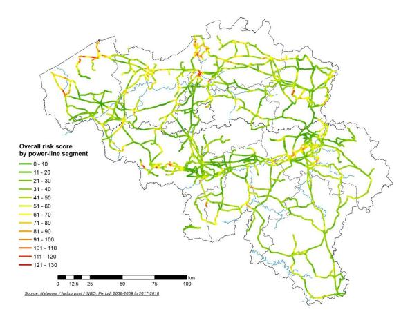
Figure 17: Map of the current Elia grid of power lines (including sections owned by other parties but managed by Elia). Sections are colour-coded based on their collision risk scores. Most of the high-priority lines are close to waterbird sites, with a higher risk clearly existing in the polders area and the Yser valley and the lower Scheldt valley, and in Wallonia around the Harchies marshes and the lower Meuse valley.
